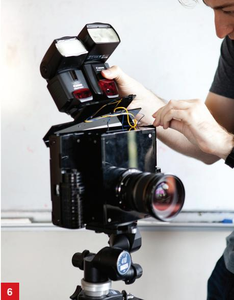
**6.** David Jacobs, one of the graduate students working on Marc Levoy's project, prepares for an experiment by attaching a top plate with two hot shoes, used to mount and control flashguns. Conventional cameras can control multiple flash units, but they can be triggered only once, simultaneously, during an exposure. The Frankencamera can be programmed to set off up to eight flashguns at different times during a shot.
