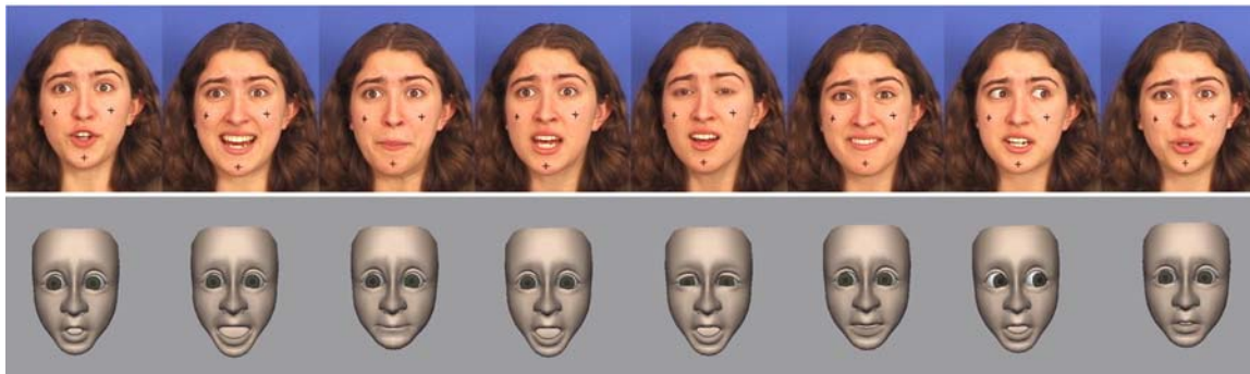
Figure 8(b): Example frames from another sequence retargeted onto the same 3D face model. This sequence uses a new set of key shapes that better match the range of expression that exists in this sequence.
