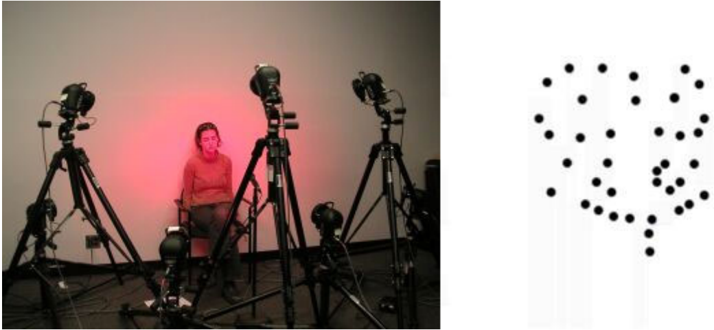
Figure 3.12: Marker-based motion capture. On the left: 7 cameras set up with the Vicon system. On the right: the facial markers.
