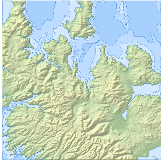
Figure 1: Medium-scale map with hill shading and low-detail bathymetric contours, all generated automatically.
