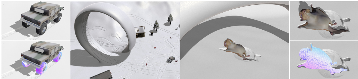
Figure 1: Example scenes showing our real-time surface deformation technique. The user-controlled car (left) and the animated character (right) cause fine-scale deformations on the terrain surfaces. While deformable surfaces are represented as displaced Catmull-Clark subdivision surfaces, we voxelize the actual surface geometry of rigid objects in order to determine their respective deformations.
