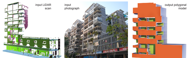
Figure 6. In case of poor quality input and insufficient repetitions, we may fail to identify variations among repeated elements, e.g., different potted plants and railings across balconies. As a result, the final polygonal model incorrectly contains identical balconies.
