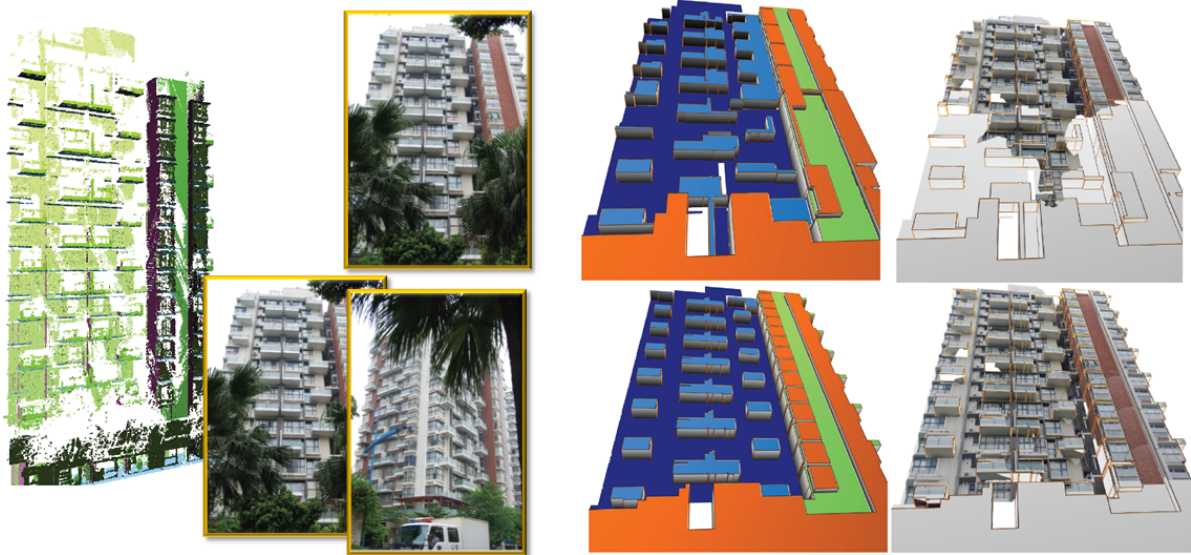
Figure 8. Photographs can have significant parts occluded due to trees and other obstacles (top row). The occlusions, however, are usually different across views thus resulting in improved geometry and texture consolidation when we use more images. In this example we added another photograph from a different view to significantly improve the resulting 3D model (bottom row).
