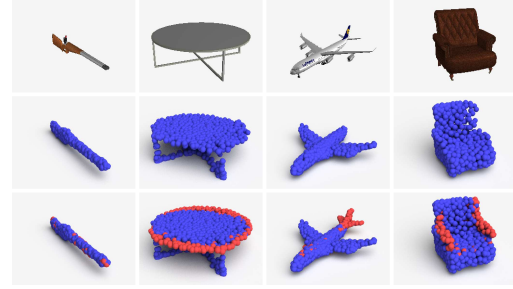
Figure 10. Visualization of points predicted by the deconvolution branch (blue) versus the fully connected branch (red).
