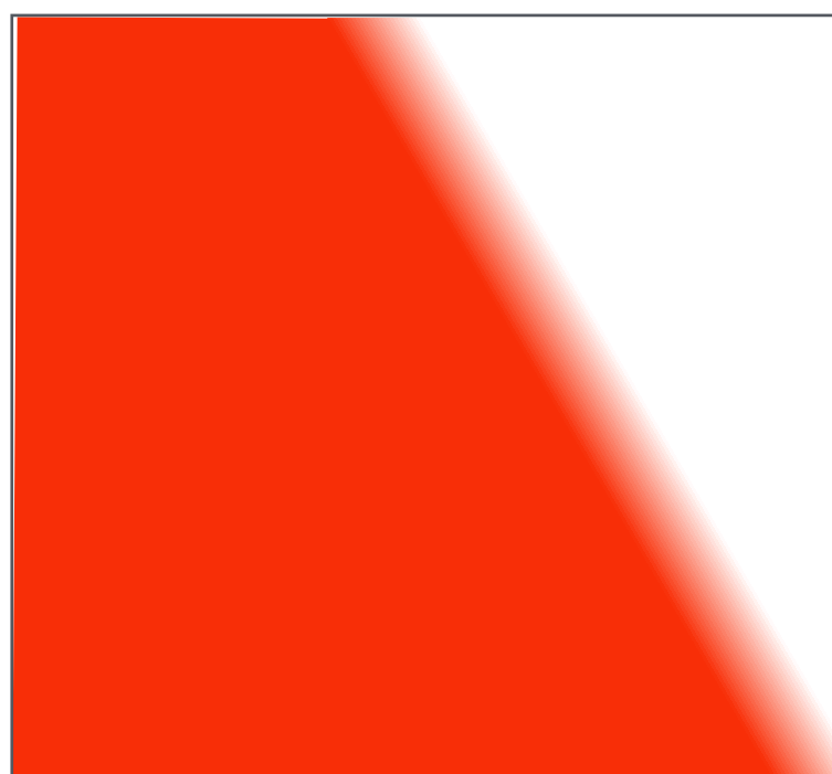
Reconstructed signal (averaging over pixel (via convolution) yields new signal with high frequencies removed)
