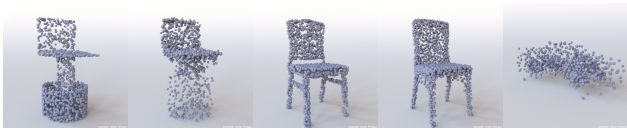
Figure 19. The AEs might fail to reconstruct uncommon geometries or might miss high-frequency details: first four images - left of each pair is the input, right the reconstruction. The r-GAN may synthesize noisy/unrealistic results, cf. a car (right most image).
