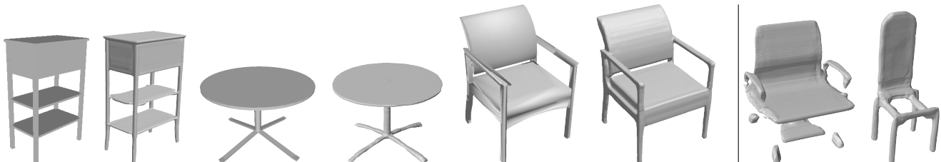
Figure 7: Reconstruction of test shapes. From left to right alternating: ground truth shape and our reconstruction. The two right most columns show failure modes of DeepSDF. These failures are likely due to lack of training data and failure of minimization convergence.
