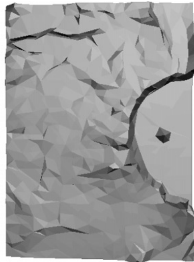
Figure 13: Simplified model with 999 faces (took 46 seconds).
