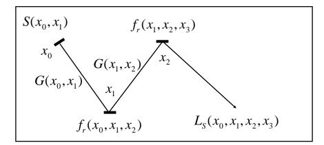
$$L_{S}(x_{0}, x_{1}, x_{2}, x_{3}) = S(x_{0}, x_{1})G(x_{0}, x_{1})f_{r}(x_{0}, x_{1}, x_{2})G(x_{1}, x_{2})f_{r}(x_{1}, x_{2}, x_{3})$$
