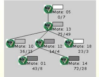
Example: ad hoc, multi-hop routing of photo sensor readings
