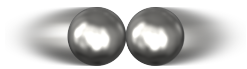
Figure 2: Small ball bearings vibrate too quickly to produce audible modal sound. Instead, their sound is the result of rigid acceleration experienced during collisions.
