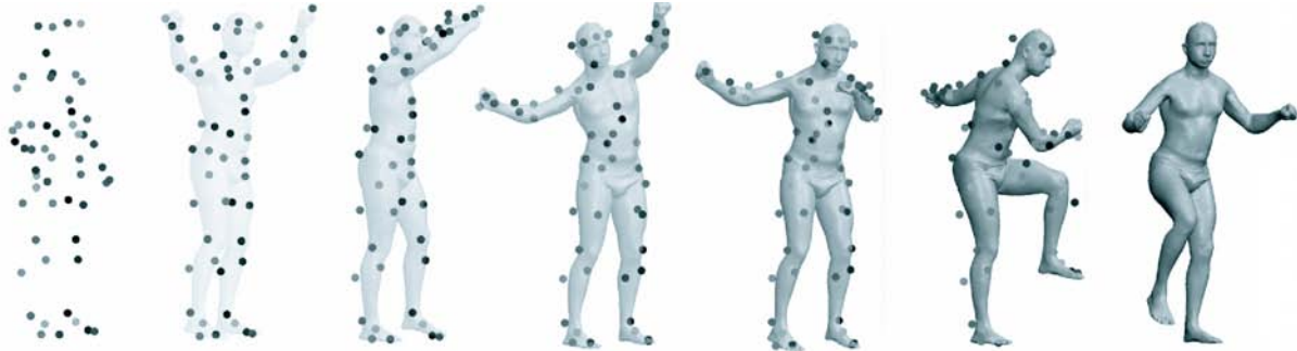
Figure 1: Animation of a motion capture sequence taken for a subject, of whom we have a single body scan. The muscle deformations are synthesized automatically from the space of pose and body shape deformations.
