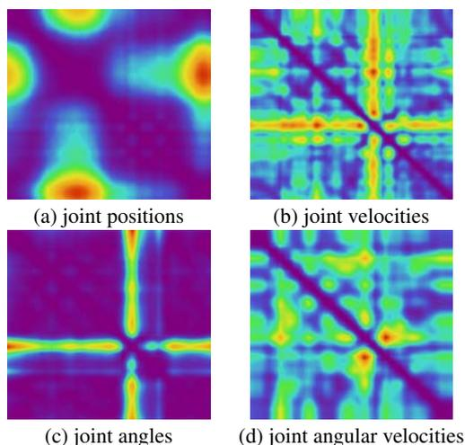
Figure 4: The four affinity matrices. Each matrix captures the dissimilarity among the poses aspects. The different contribution of each aspect is evident from the differences in the location of most dissimilar poses.
