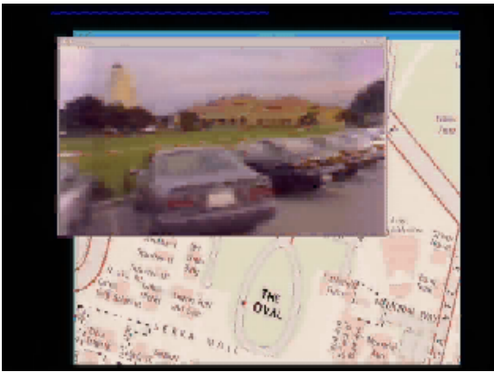
Figure 8: This image shows a single frame from the video panorama project. The video panorama consists of a tour of Stanford campus. At each point in time a full 360 degree panorama is received and the user is free to browse around, but a default view is provided. The display also shows a map of the campus with a pointer indicating the current position. By clicking on a location on the map the current viewing direction rotates and locks onto this feature allowing a user to watch it while the tour continues.
