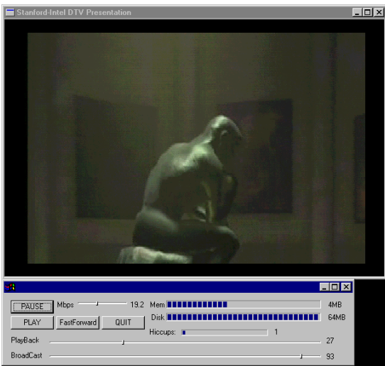
Figure 3: A screen shot of the Virtual VCR, where the top window shows the decoded video. The bottom window shows the control panel, the current memory and disk usage, and the reception and decoding progress.
