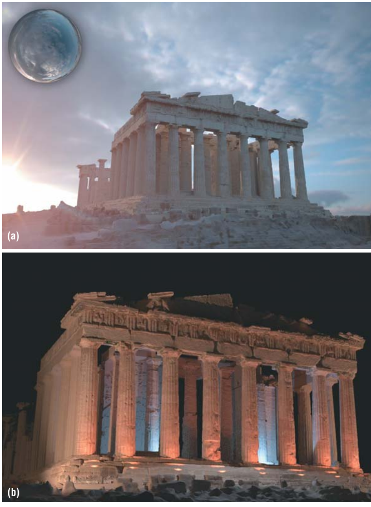
Figure 8. The Parthenon virtually reilluminated. (a) A virtual model of the Parthenon rendered as it would appear under natural illumination (inset) recorded in Marina del Rey, California. (b) The relightable model rendered with a nighttime lighting design.
