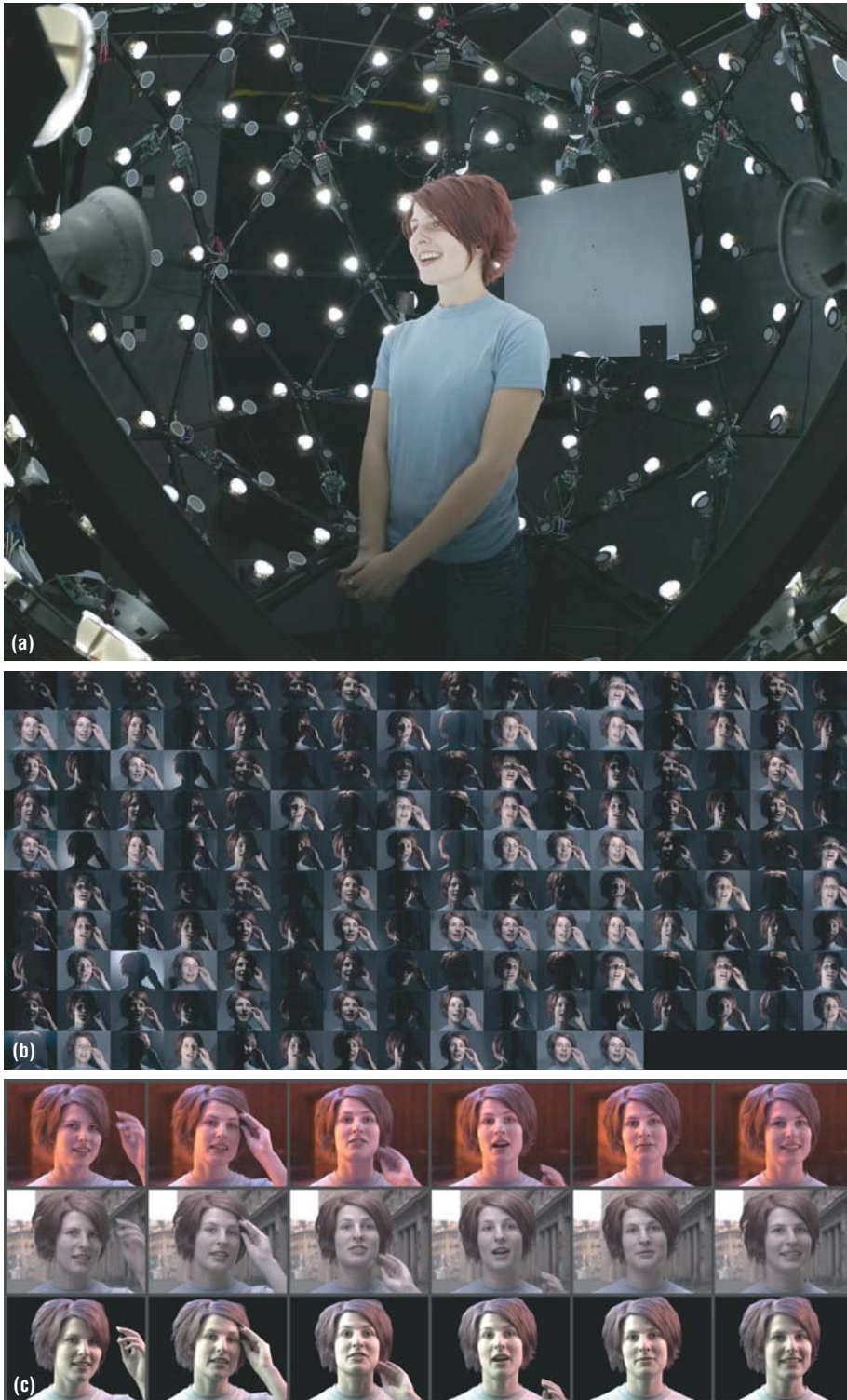
Figure 3. The Light Stage 5 performance relighting process. (a) A sphere of 156 white LED light sources surrounds the actor as a microcontroller changes the lighting direction several thousand times per second. A high-speed digital video camera captures the actor's appearance under each lighting direction. (b) 156 consecutive high-speed frames of the actor's performance captured in just 1/24th of a second, each showing a different basis lighting direction. (c) The actor's performance synthetically illuminated by two real-world lighting environments (Grace Cathedral, top; the Uffizi Gallery, middle) and a synthetic lighting environment (below) formed as linear combinations of the basis lighting directions.
