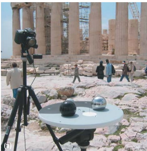
Figure 7. Capturing the lighting and geometry of the Parthenon. (a) A light probe device records incident lighting conditions near the base of the temple. (b) A 3D surface model of the scene geometry obtained using 3D laser scanning.
