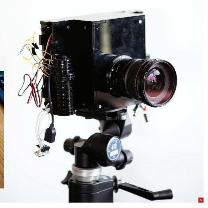
1. The Frankencamera's case is carved from sheets of acrylic plastic using a laser cutter, following a design stored on a computer. Large sections are cut out to make the case's main panels; smaller pieces are glued into stacks to make some parts, such as the camera's grip.
