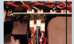
Connectors converge on the main processor's circuit board.
