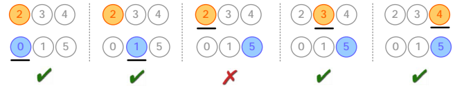
Figure 4: Step-by-step execution of the example given above. Cuts are shown by their node indices: 2, 3, 4 for the orange cut; 0, 1, 5 for the blue cut. Shaded nodes are the current nodes in execution; underscore marks the smallest index at each step; checkmarks indicate whether the nodes overlap or not.
