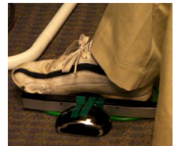
Figure 2: SlideMouse + Optical Sensor Prototype
