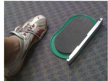
Figure 1– the SlideMouse: plastic slider + IR emitter]
