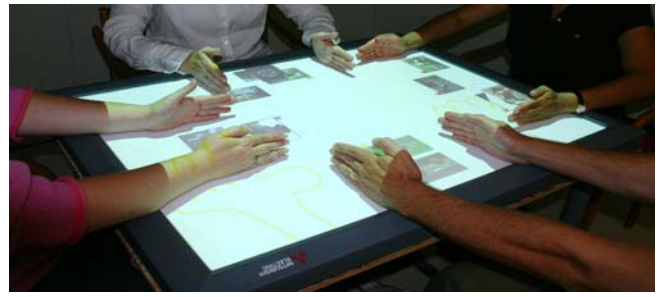
Figure 6. When all four group members simultaneously perform the “neaten” gesture, the result is to organize all of the photos on the table into a single, central pile.
