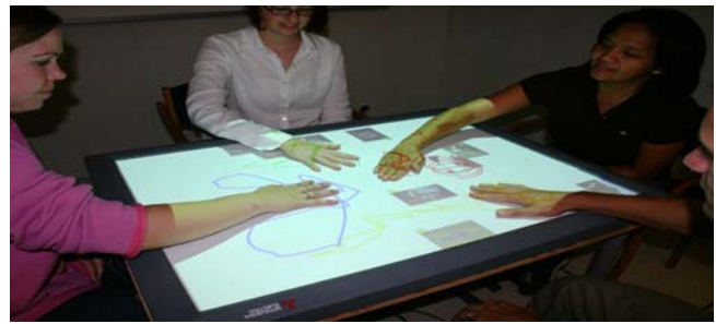
Figure 2. When all group members simultaneously “erase,” the “clear screen” action is invoked.
