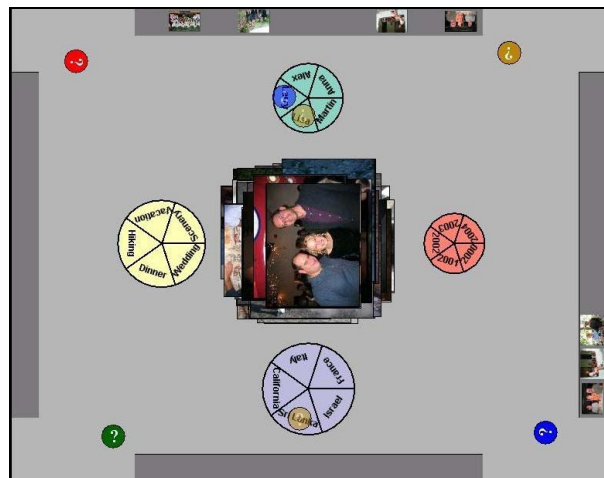
Figure 4. TeamSearch with parallel query tokens : each group member's tokens (distinguished by color) form distinct queries.
