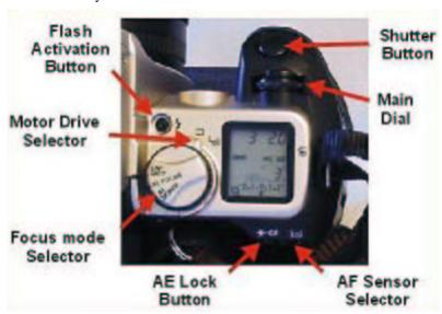
Figure 3: Focus Mode Switch
