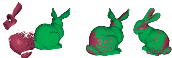
Figure 5: Partial Match: A partial scan of the bunny (shown in purple) is registered to the bunny, the model PCD. The initial arrangement of the PCDs is shown to the left. Our algorithm found the correct match (middle, right) in six iterations.
