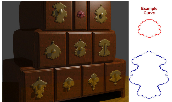
Figure 9: From a simple sketch of the handle of a cabinet, several complex cabinet handles are designed automatically in the same style. The example handle is the top center red-tinted handle.
