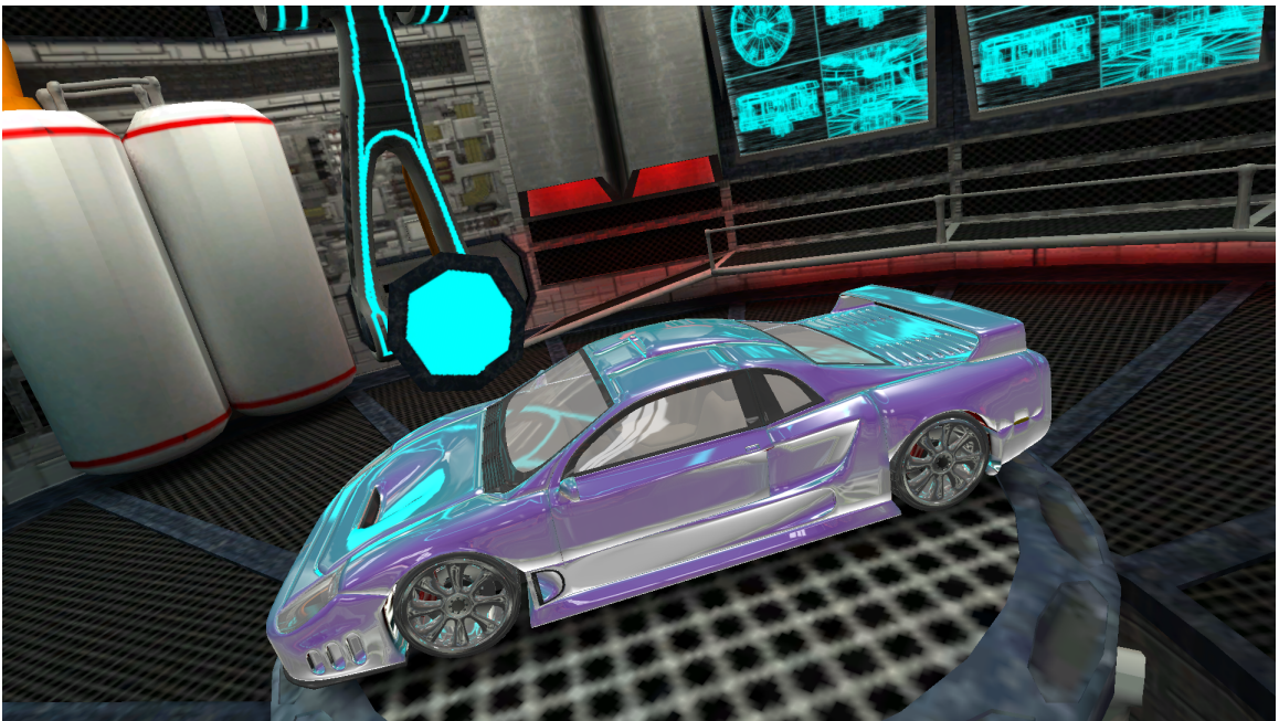
Figure 4.5: CubeMapGS example, showing a car model reflecting its environment, using a dynamic reflection cube map.
