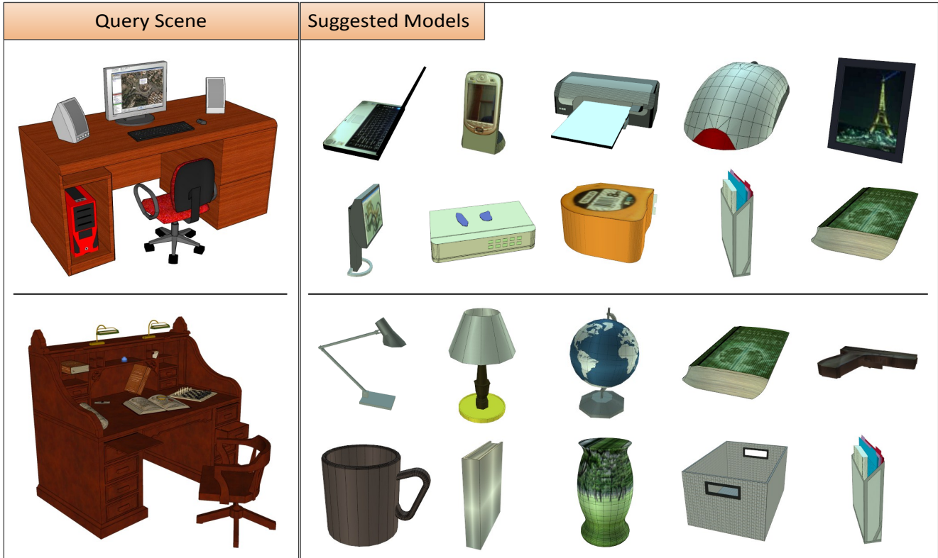
Figure 8: Context-based model search results. Left: A user modeling a desk scene issues a query for a model to be placed on the desk. Right: Highest ranked models for each query. Note how the context provided by the models in the query scene influences the categories of the suggestions.
