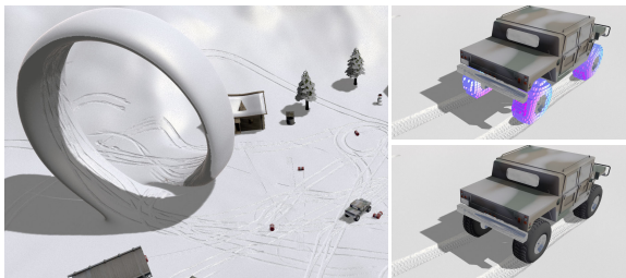
Figure 22: Examples of real-time deformation method with fine-scale surface deformations on object collisions. The tracks of the car and barrels (left) are generated on-the-fly by updating the surface displacement map using a voxelization of the colliding objects as the user controls the car.
