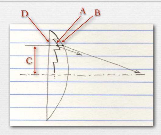
each Fresnel segment (A) is roughly parallel to that part of the original lens (B) which is at the same ray height (distance from the optical axis (C)), but it's closer to the planar surface (D), making the lens physically thinner, hence lighter and cheaper
