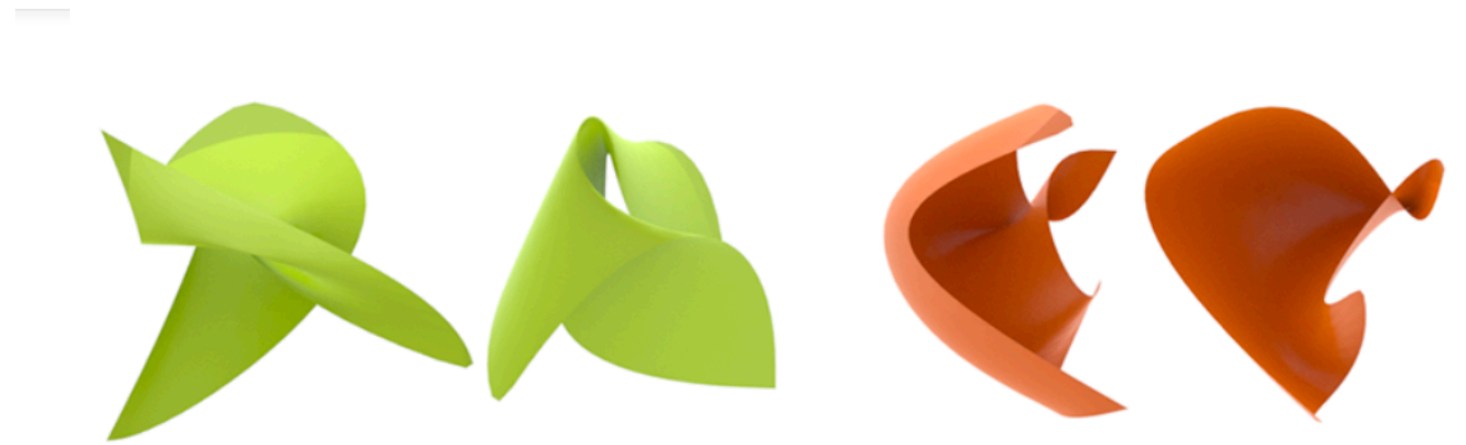
Fig. 5. Example patches misclassified by the self-intersection MLP. Two false positives (incorrectly predicted to be self-intersecting) are shown in green, and two false negatives are shown in orange.
