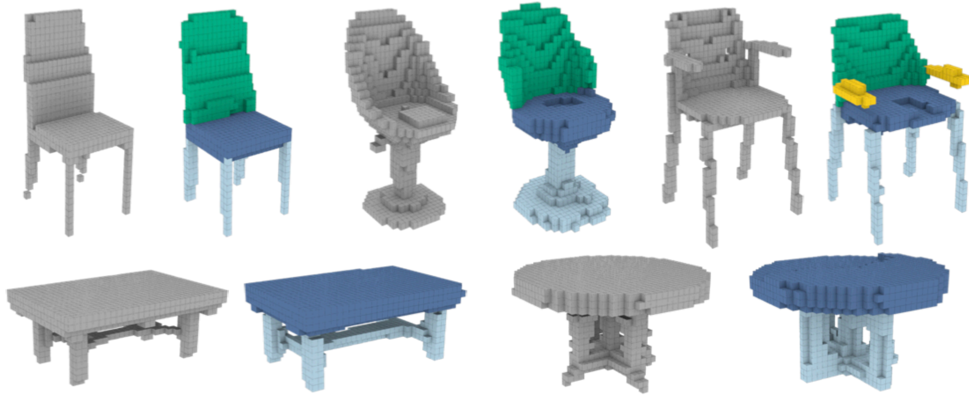
Figure 4: Reconstruction results of the proposed pipeline, for chair and table shapes. Gray shapes are the input test shapes; the results are colored according to the part label.
