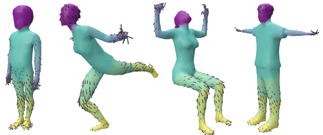
Fig. 8. Vector-valued featuremap and label predictions from our Harmonic Surface Network trained on shape segmentation.
