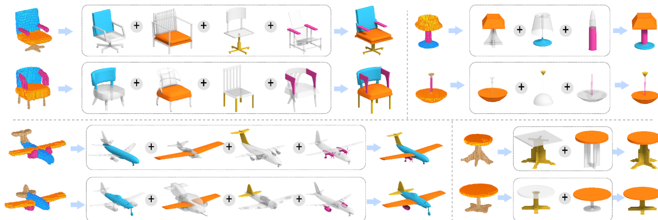
Fig. 10. Part-wise surface assembly. We present two examples for each category. On the left column is our generated shape, in the middle columns are the part-wise nearest neighbors from the training set. On the right column is our reconstructed mesh that fits the generated shape.
