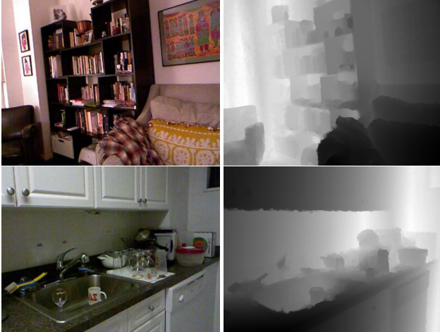
Figure 6: Two examples of RGB-D images from the NYU Depth dataset (v2) [16]. Each example comprises an RGB image (left) and a corresponding depth image (right).
