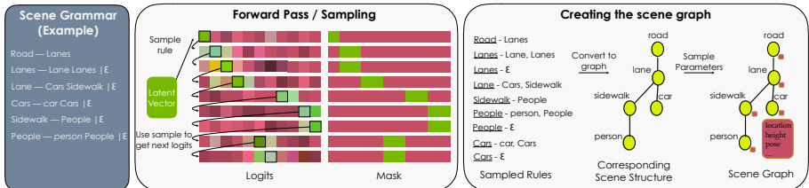
Fig. 3. Representation of our generative process for a scene graph. The logits and mask are of shape T_{max} \times K . Green represents a higher value and red is lower. At every time step, we autoregressively sample a rule and predict the logits for the next rule conditioned on the sample (capturing context dependencies). The figure on the right shows how sampled rules from the grammar are converted into a graph structure (only objects that are renderable are kept from the full grammar string). Parameters for every node can be sampled from a prior or optionally learnt with the method of [30]. A generated scene graph can be rendered as shown in Fig. 2.
