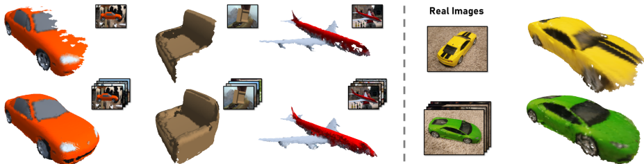
Fig. 1. Pix2Surf learns to generate a continuous parametric 3D surface of an object seen in one or more views. Given a single image, we can reconstruct a continuous partial 3D shape (top row). When multiple views are available, we can aggregate the views to form a set of consistent 3D surfaces (bottom row). Our reconstructions preserve 2D pixel to 3D shape correspondence that allows the transport of textures, even from real images (last column).
