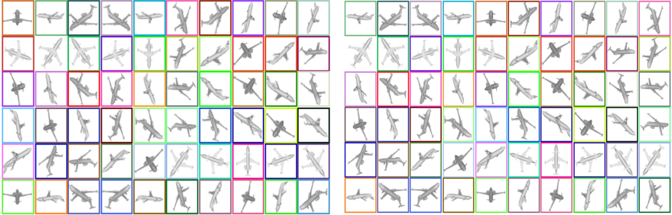
Figure 7: Equivariance of view configurations to \mathcal{I} . The views on the left and right are obtained from 3D shapes separated by a 72 deg rotation in the discrete group. We mark corresponding views before and after rotation with same border color. Notice the five first views in the second row – the axis of rotation is aligned with their optical axis; the rotation effect is a shift right of one position for these views. It is clear that when g \in \mathcal{I} is applied to the object, the views are correspondingly permuted in the order given by the Cayley table, showing that the mapping from 3D shape to view set is equivariant.
