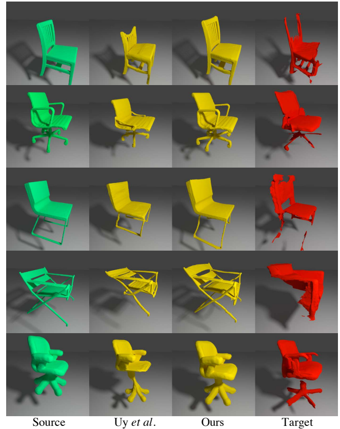
Fig. 13. Fitting errors between retrieved/deformed CAD models and scans in Scan2CAD [Avetisyan et al. 2019a]. Our deformation produces results that are more visually appealing with smaller fitting errors, compared to the state-of-the-art.
