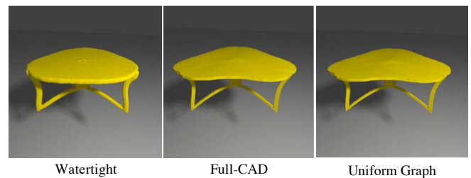
Fig. 7. Deformation results with different mesh representations. Although watertight approximation [Huang et al. 2018a] can achieve good fitting to the target, the geometry is different and sharp features can not be well-preserved. Our skeleton template representation is a good approximation which generates quite similar results comparing with direct optimization of the original CAD model.
