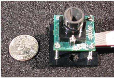
Figure 2: Our camera tiles contain an Omnivision 8610 image sensor, passive electronics, and a lens mount. The ribbon cables carry video data, synchronization signals, control signals, and power between the tile and the processing board. To keep costs low, we use fixed-focus, fixed-aperture lenses.
