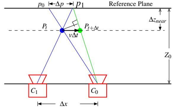
Figure 8: The temporal and spatial view axes are related by image motion. For a given scene configuration, we can determine a time step  $\Delta t$  for which the maximum image motion between temporal samples is equal to the maximum parallax between spatially neighboring views. If we measure time in increments of  $\Delta t$  and space in increments of the camera spacing, then the Manhattan distance between view coordinates corresponds to the maximum possible image motion between views.
