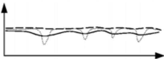
**10** The dotted curve is the true surface; it's coarsely approximated by a B-spline surface, shown with the solid curve. But to approximate the virgin (unmarked) surface, we really want the alpha hull, drawn with the dashed curve. The difference between this curve and the true surface curves represents the inscriptions better.
