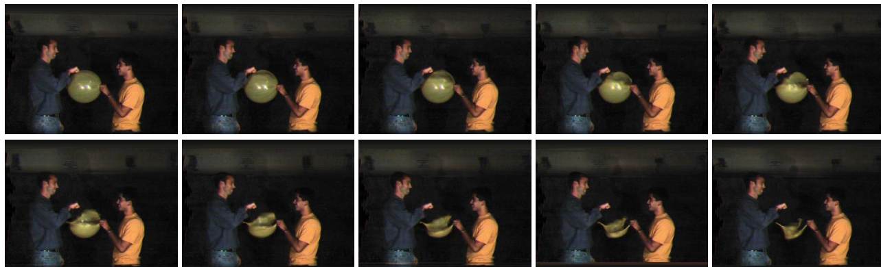
Figure 10: 1560fps video of a popping balloon, corrected to eliminate rolling shutter distortions.
