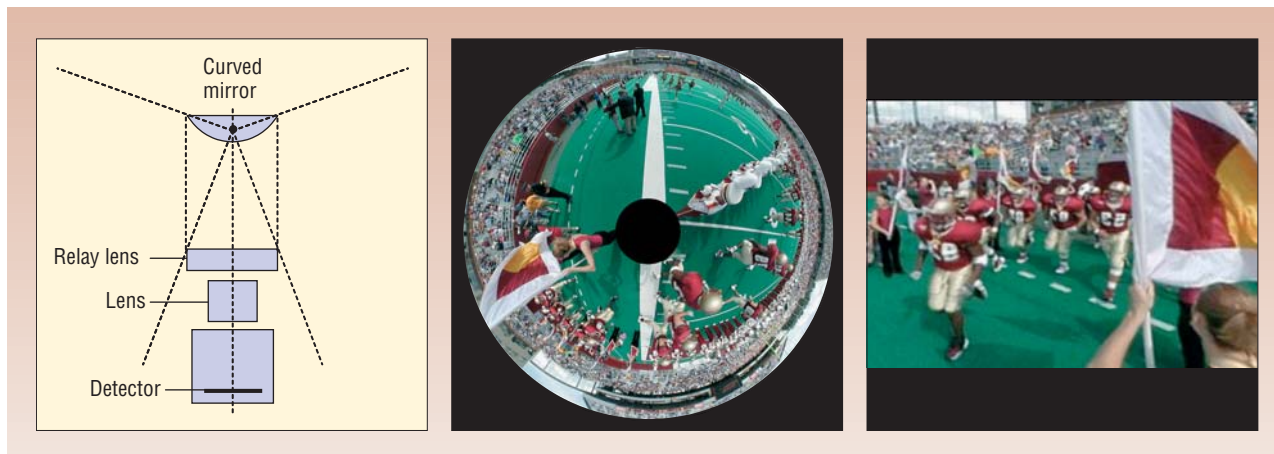
Figure 2. Wide-angle imaging using a catadioptric camera.
