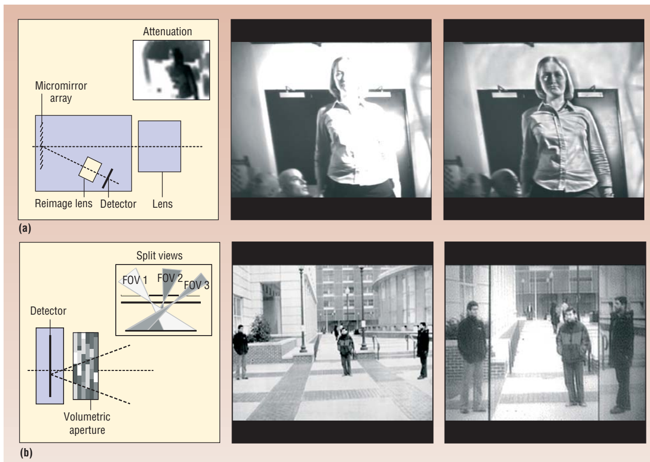
Figure 7. Programmable imaging systems that use controllable spatial light modulators to vary their radiometric and geometric properties based on the application's needs. (a) Adaptive dynamic-range imaging with a micromirror array. (b) Split field-of-view imaging with a volumetric aperture.
