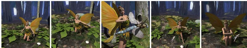
Fig. 1. Screenshots from an animated 180,000 triangle scene with moving dragonfly, fairy, and plants. At  $1024 \times 1024$  pixels the animated scene is ray traced at roughly 3.7 frames per second on a dual-2.6 GHz Opteron desktop PC including shadows and texturing.
