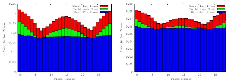
Fig. 10. Impact of BVH quality for  $2 \times 2$ ,  $4 \times 4$ , and  $16 \times 16$  ray packets (for the runner model only, other models exhibit similar behavior). Each graph shows the best and worst performance for any of the time step’s deformed BVHs, as well as the best BVH over time performance. As can be seen, the difference between best and worst BVH can be significant for small packets, but diminishes for larger packet sizes.
