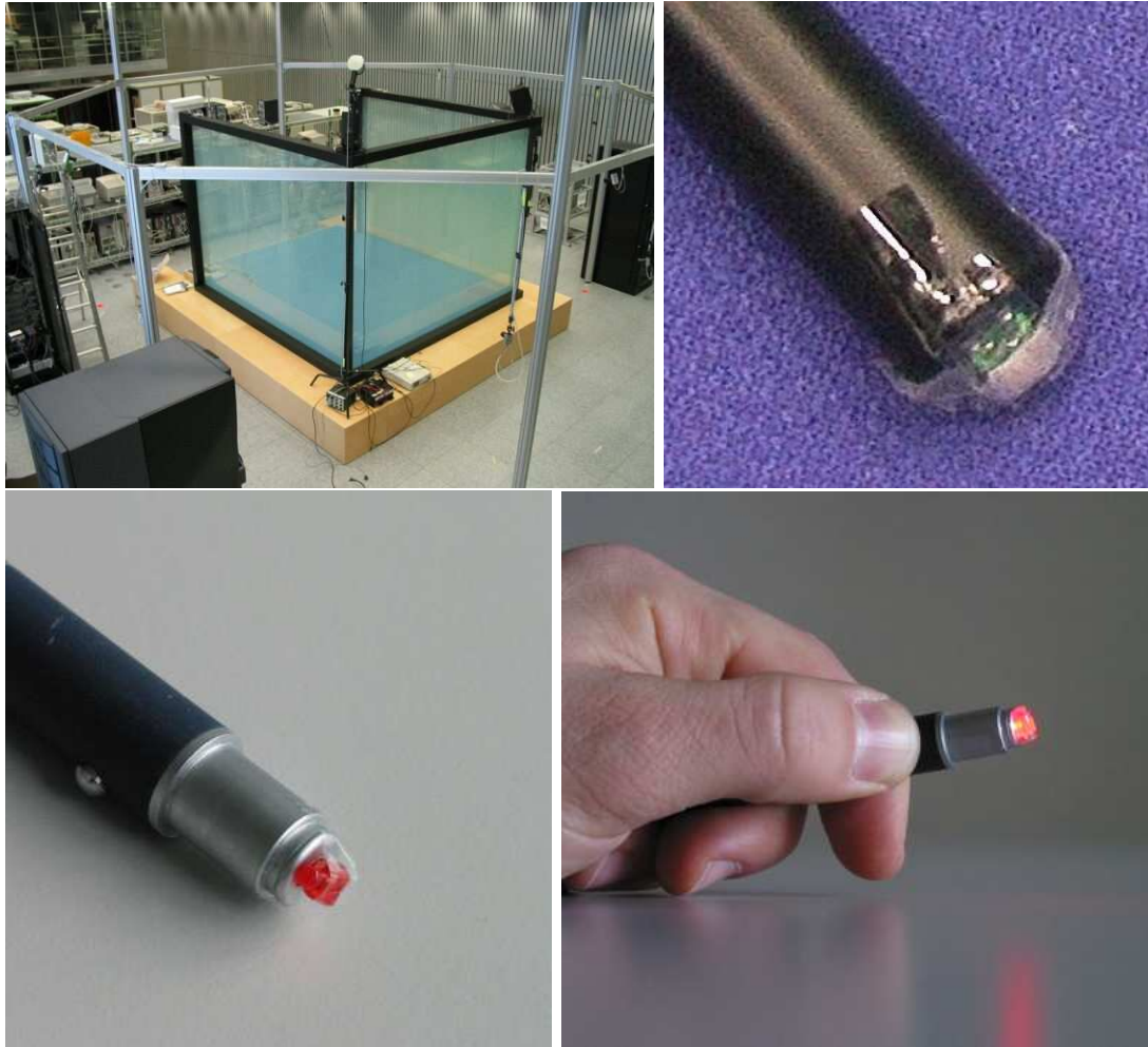
Figure 2: Immersive virtual environment BlueC [8] and the modification of a laser pointer. Small piece of transparent green or red plastic is attached to the laser pointer. The modification has been invented in order to get better visibility from different viewpoints. However primitive solution it is, it does the job very well. The working volume is inside the glass cave. Four cameras are mounted in the top four corners of the construction and the remaining 12 cameras are mounted on the aluminum scaffold that encompasses the cave.
