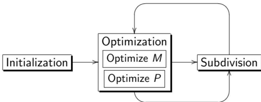
We optimize the **spatial position** of the faces of  $M$  and the **geometry** of the faces of  $P$  in an alternating fashion.
