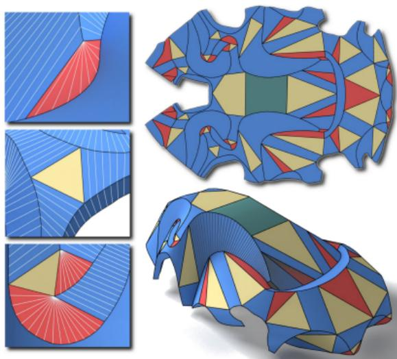
Torsal ruled surfaces can be decomposed into patches lying on
