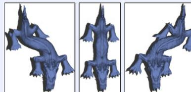
Geodesic interpolation can be used to cope with notions such as symmetry. Symmetric poses correspond to geodesic midpoints.
