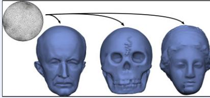
We model geometric objects – shapes – by mapping a fixed connectivity (a simplicial complex) to each object under consideration. The vertex correspondence problem is solved in an independent preprocessing step.
