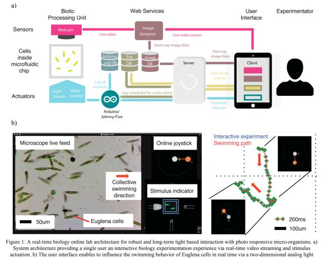
actuation. b) The user interface enables to influence the swimming behavior of Euglena cells in real time via a two-dimensional analog light stimulus applied via a joystick (right: example of change in swimming path of a single cell upon light stimulus actuated in real time by joystick).
